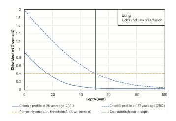
Independent third-party tests conducted on the Lascelles Wharf slabs in 2014 and 2021 confirmed the effectiveness of Xypex-treated concrete. The 2014 tests showed minimal damage, low chloride penetration, and no significant carbonation, estimating a service life of 164 years using Fick's 2nd Law of Diffusion.
